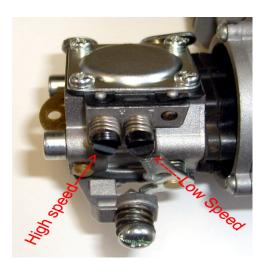
After you have the high speed needle set check the idle and transition to full throttle. If It is OK then leave it alone. If when transitioning to full throttle the engine sputters and dies then open (turn counter clock-wise) the low speed needle 1/8". Try transitioning to full throttle again, keep adjusting until you get a good transition from idle to full throttle.
